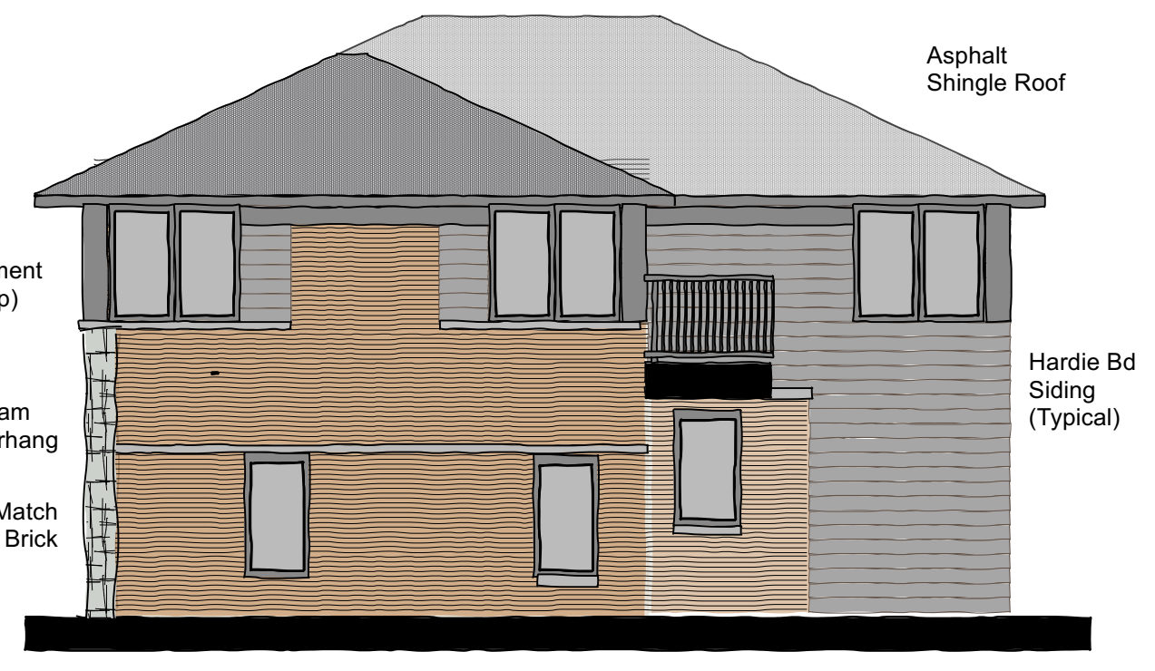
7 PROPOSED East Elevation (Street) ELEVATION = 846 SF MASONRY = 566 SF HARDIE BD = 274 SF Scale: 1/8" = 1'-0"
