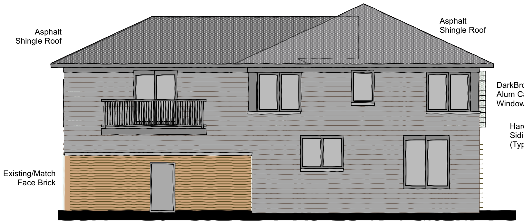
4 PROPOSED WEST Elevation (BACK YARD) ELEVATION = 846 SF MASONRY = 190 SF HARDIE BD = 656 SF Scale: 1/8" = 1'-0"
