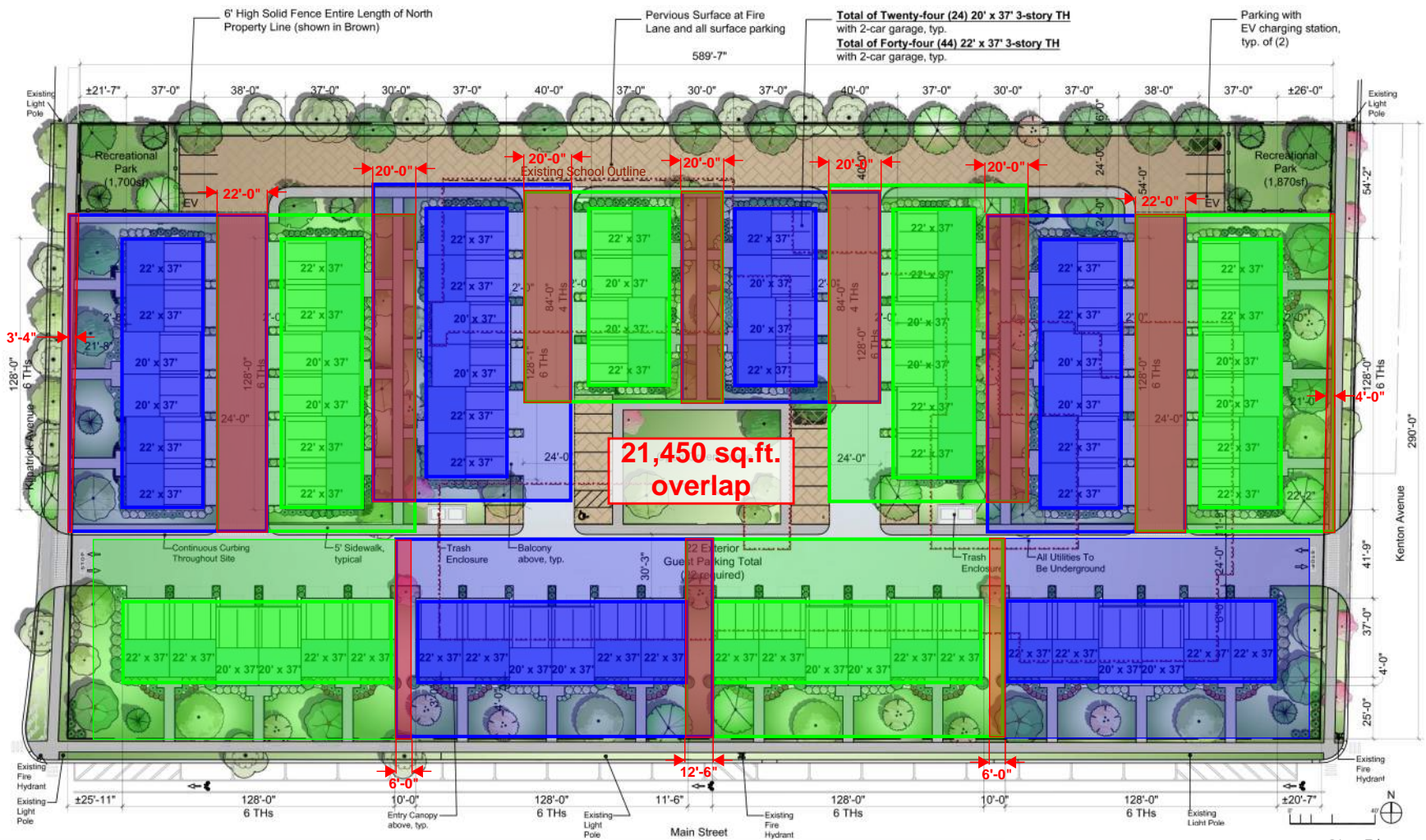
Figure 1. Site plan illustrating interference (red shading) of Code-required yard geometry (light shaded rectangles) for the twelve proposed buildings (dark shaded rectangles).
