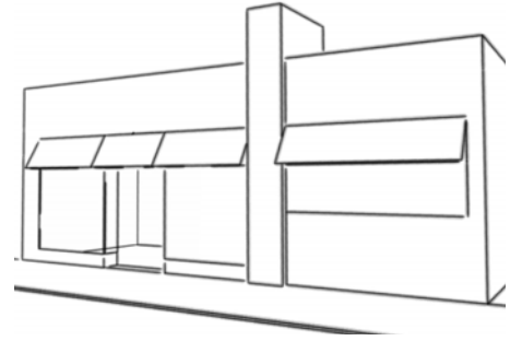
Acceptable design: awnings that frame each window and entrance but do not cover architectural features
