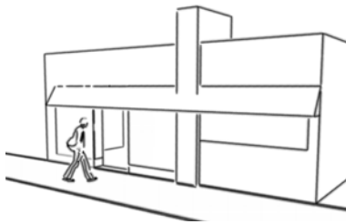
Unacceptable design: a continuous awning blocking an architectural feature.
